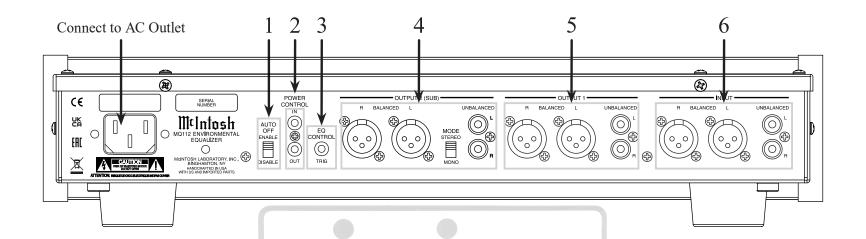
1. AUTO OFF when set to ENABLE, the unit will power itself down if no audio signal is present at the input for at least 30 minutes. When set to DISABLE, the unit will remain on until manually turned off by the user.
