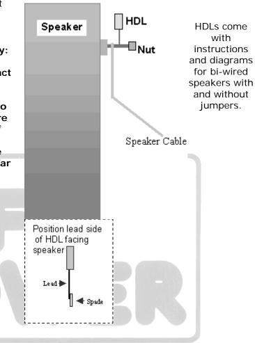
Biwireable Speakers - Using one set of speaker cables with jumpers: You will need one pair of HDLs and one pair of jumpers. The jumper wire is critical. We recommend our Walker Audio Silver Jumpers. They are cryogenically-treated ultra-pure silver solid-core jumpers. Your ears will love you.
