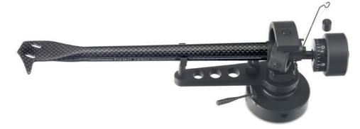
The tonearm's design efficiently leads parasitic vibrations away from the cartridge into the mounting board, guarantees the precise tracing of the record groove by the needle and also facilitates fine adjustment of vertical and horizontal tracing due to the following constructional details:
