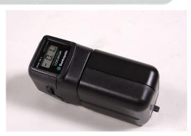
The Sunhayato EG-5 static electricity meter is small and very easy to use. The result is displayed on the display directly in kV.
